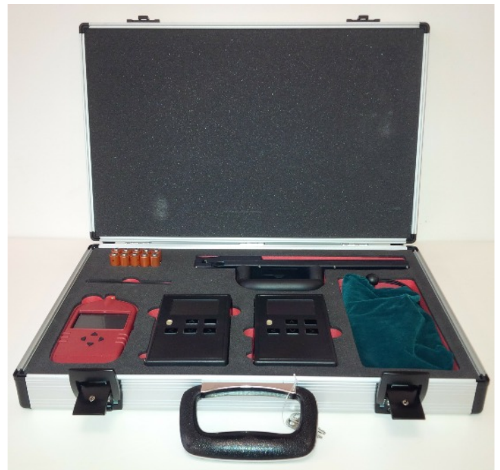
L-R: Lockhart RF, Conducted Signals, Optical. Top: Surface Scanner
